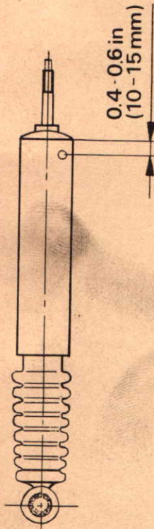
PNEUMATIC SHOCK ABSORBER WITH RUBBER BELLOWS, GAS CHAMBER AT TOP
